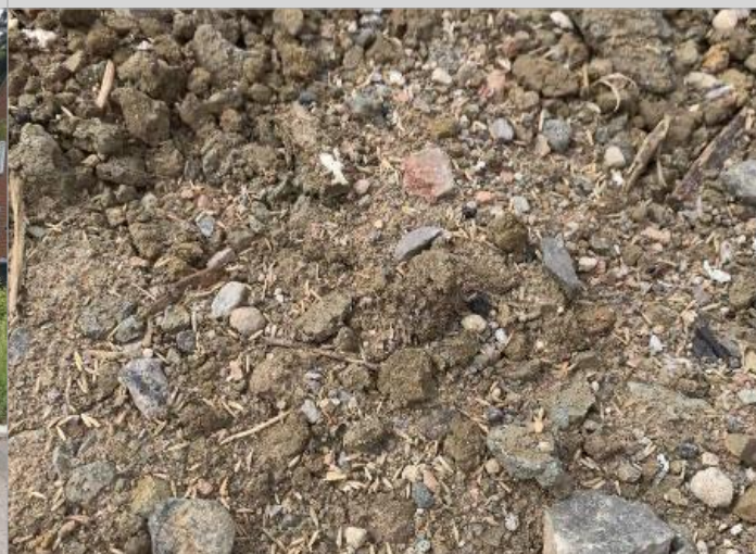
BOVIS - Poor quality of final topsoil for verges
